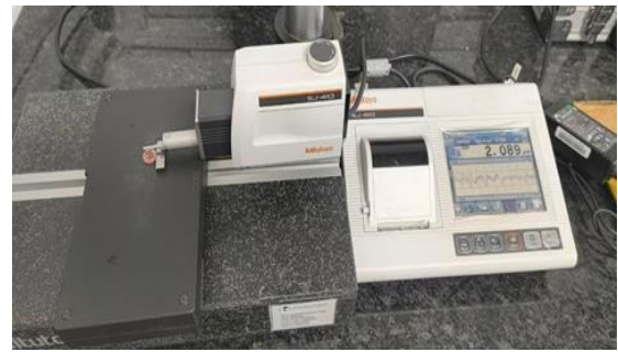
Figure 5: Surface roughness evaluation set up
